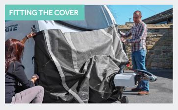
Insert the TOW PRO LITE into the awning channels on either side of the caravan - the same way you would do an awning. Slide the cover either up or down the channels, depending on your opening's location, until it sits neatly on the A-frame section.
